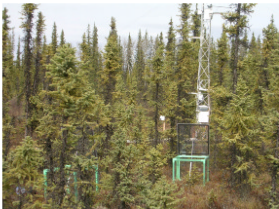
Photo. 1 Automated soil CO 2 efflux chambers at the CO 2 flux site of the University of Alaska Fairbanks (UAF).
